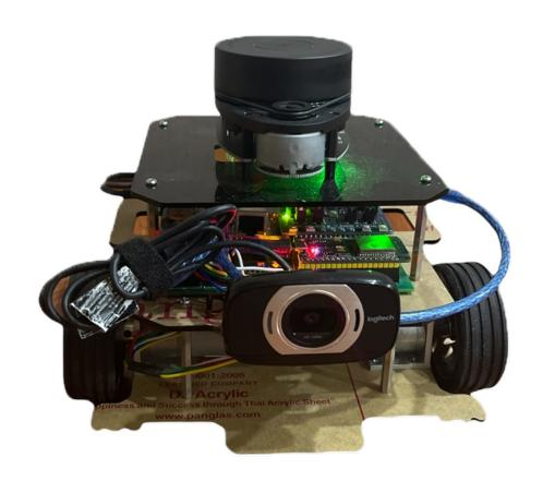
Yarm bot is an implementation of the kaebot system. Yarmbot is a guard robot that include a webcam and can detect human face. It will walk around a path every hour and you can see the live stream from your computer and mobile phone.
